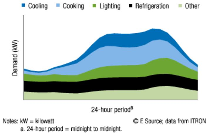
Figure 3. Example of load disaggregation for a commercial restaurant<sup>15</sup>
